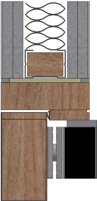
*Outward opening using flat mounting plate
