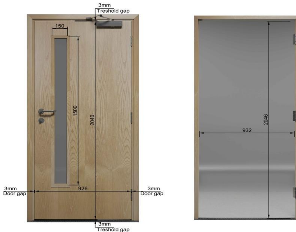
Figure 1: Dimensions of door and required door frame
