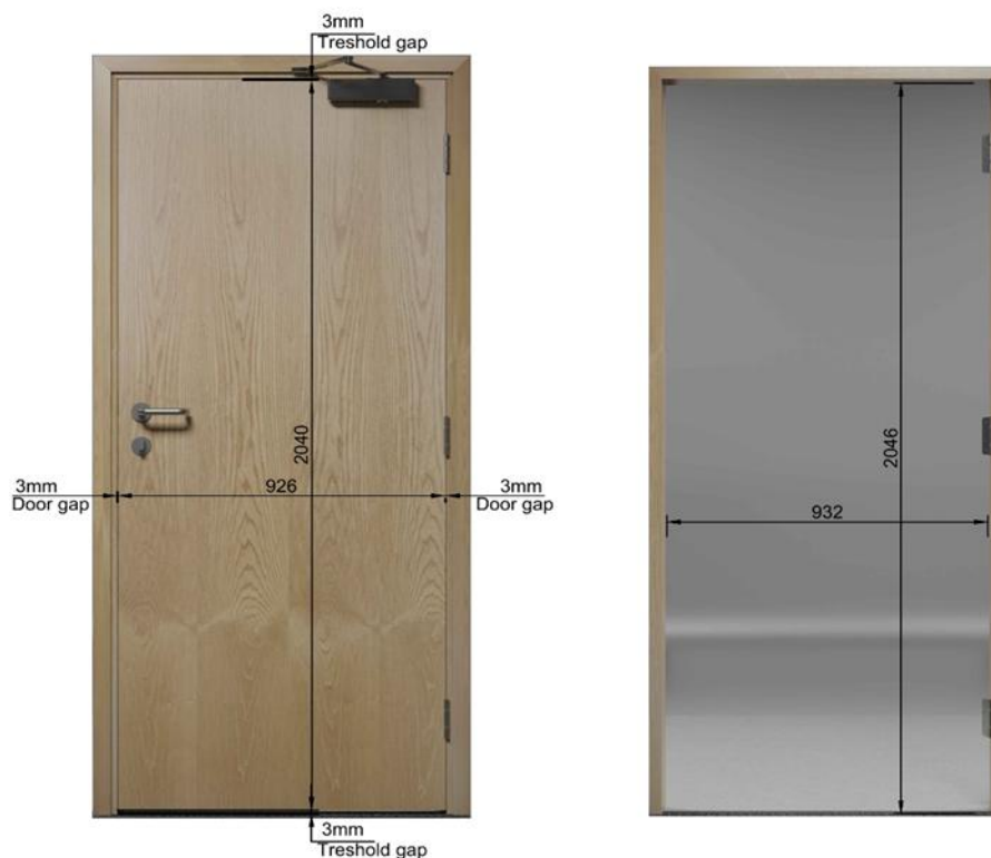
Figure 1: Dimensions of door and required door frame
