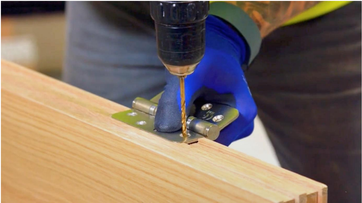
Figure 4: Generic example of fitting the hinges
